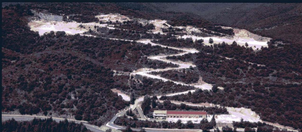
*On the same production site (40 ha), four quarries for 7 different colours. A permit to extract 45 000 tonnes per year allows close monitoring, both qualitatively and quantitatively. The techniques used are the most modern: sawing with 360° cutter and cutting with diamond wire. These techniques, combined with the expertise of our team, ensure the extraction and selection of the finest blocks.*
